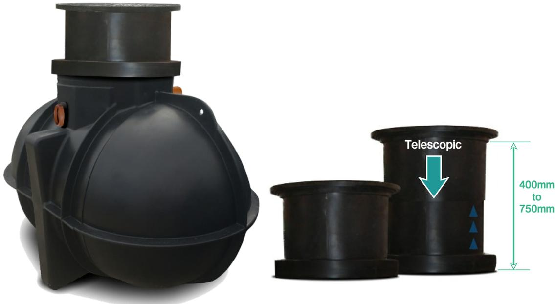
Extension risers are available for all the units (as shown above). These accommodate the respective access and access cover and can be cut to desired length with a standard saw. We recommend no more than 1000mm of extension is used via extension risers. For deeper inverts use prefabricated concrete rings or sections
